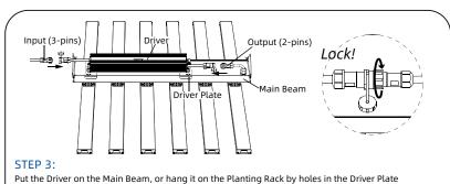
(need to customize the length of the output cable), then connect and lock the output and input
