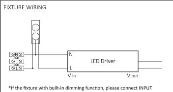
POSITIVE(+) signal conductor to DIM+ (PURPLE WIRE), INPUT NEGATIVE(-) signal conductor to DIM-(GREY WIRE) of LED driver.
