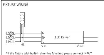
\*If the fixture with built-in dimming function, please connect INPUT POSITIVE(+) signal conductor to DIM+ (PURPLE WIRE), INPUT NEGATIVE(-) signal conductor to DIM-(GREY WIRE) of LED driver.
